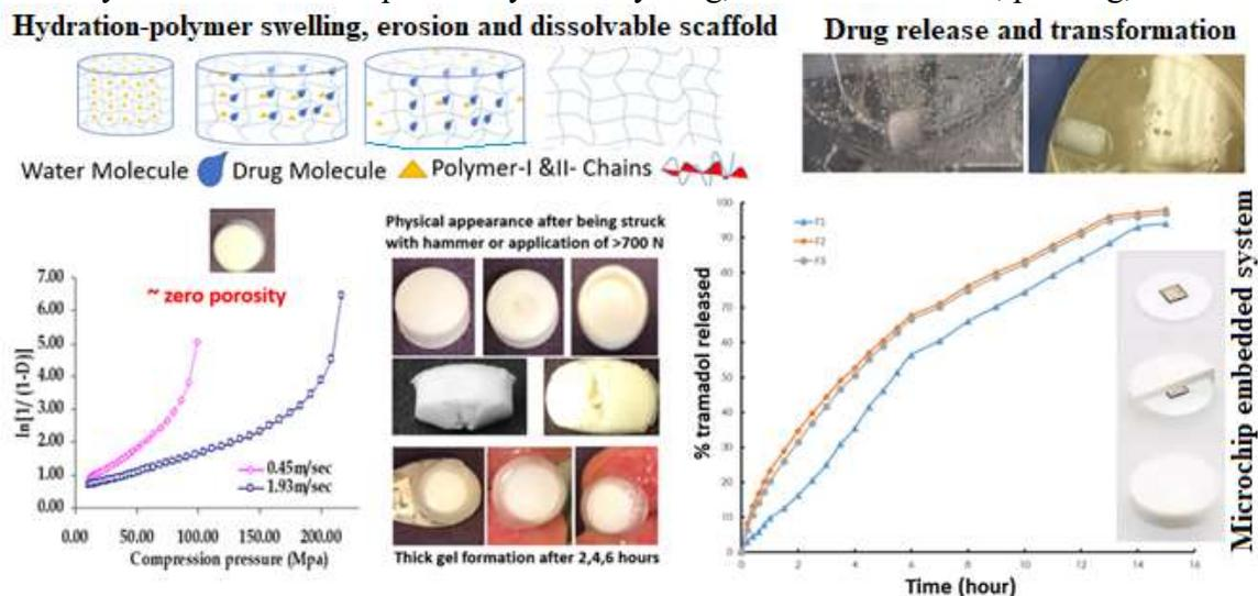
**Figure 4.** Heckel plots for Tramadol-PEO:P-II (4:1) matrices and changes in the physical appearances upon exposure to water, dissolution studies and hardness testing to demonstrate tamper-resistance properties. (US Patent Application Pending; Abuse deterrent delivery system - C2019-008). (C2019-008- International Publication Number- WO 2020/081762 A1).
