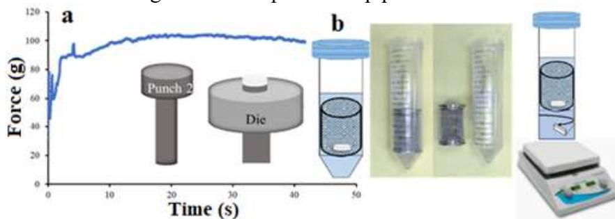
**Fig.2.** (a)-Schematics of the in-situ gel disk preparation for shape control using a mold assembly with application of 100 g force observed for highly viscous SC or IM injectable formulations, (AAPS PharmSciTech, Feb, 20, (2018). (b)-Use of USP basket fitted in tube(s) method for full surface exposure and in-situ quantification using shaker or magnetic stirrer; (AAPS-2019 & J. Pharm. Pharmacology 2020).
